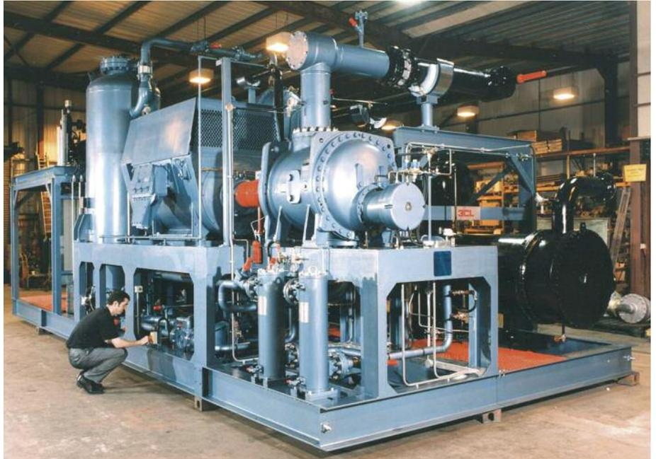
ALL WRV RANGE COMPRESSORS ARE OF DOUBLE WALL CONSTRUCTION AND UTILISE WHITE METAL, SLEEVE TYPE JOURNAL BEARINGS WITH PRESSURISED SHAFT SEAL.
